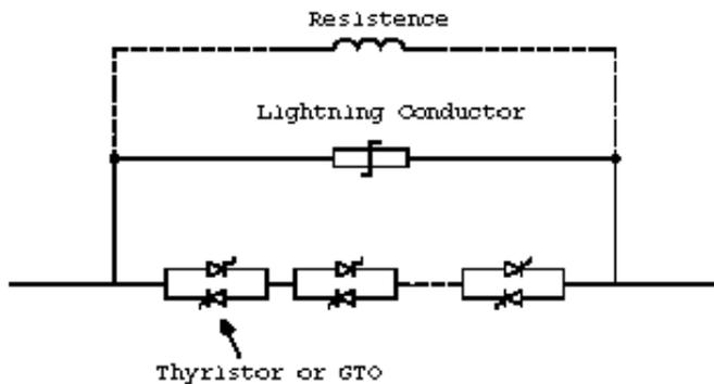
Figure 3- 19: Schematic representation of the SSB as a custom power device
