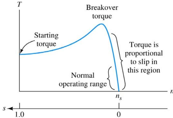
Figure 3-26: Torque speed characteristic [13]
