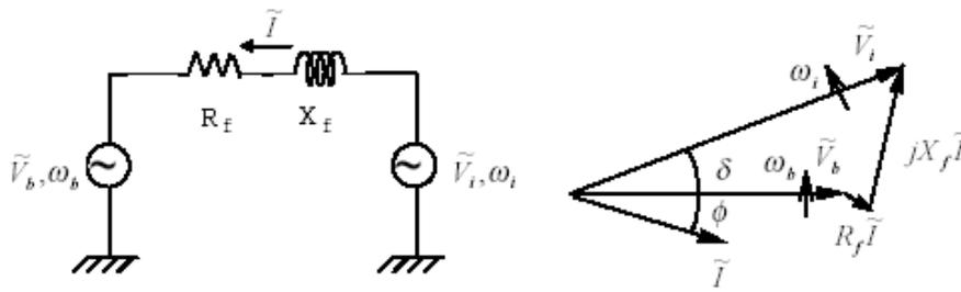
Figure 4-24: Fundamental frequency equivalent circuit and phasor diagram for the output converter
