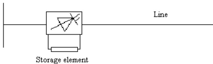
Figure 3-2: Connexion of a FACTS series controller
