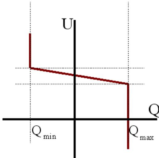
Figure 2-1: Q vs. U dependence in generator bus
