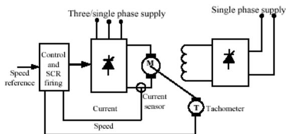
Figure 3-25: configuration of a line-frequency controlled rectifier
