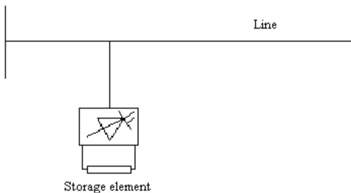
Figure 3-7: Connexion of a shunt-connected controller
