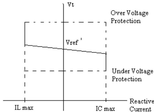
Figure 4-25: V-I<sub>Q</sub> characteristic for a renewable energy source connected to the grid through a VSC
