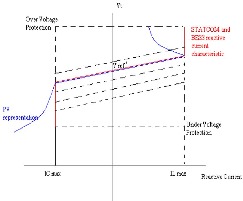
Figure 4-16: V-I reactive characteristic for a BESS and a STATCOM
