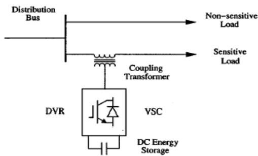
Figure 3-17: Schematic representation of the DVR for a typical custom power application
