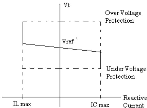
Figure 4-17: V-IQ characteristic according to the load flow convention of signs
