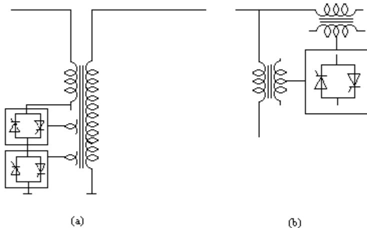
Figure 3-12: TVR (a) regular transformer with controlled tap changers
