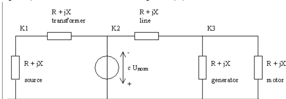
Figure 2-3b: Short circuit calculation according to IEC-909
