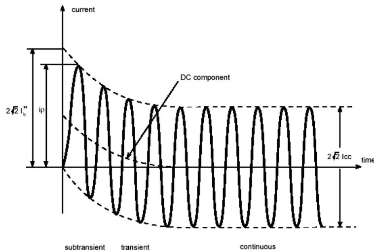
Figure 2- 2: Current evolution in a symmetrical fault
