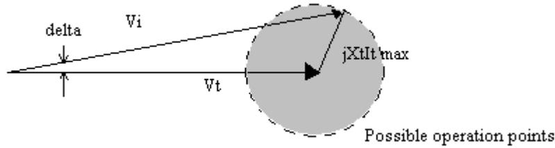
Figure 4-15: Phasor Diagram of the BESS
