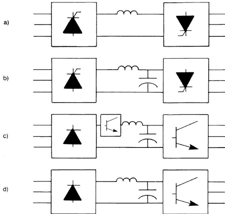
Figure 3-28: Most used configurations of AC/DC/AC converter for motor drives;
