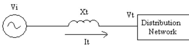
Figure 4-14: BESS equivalent Circuit
