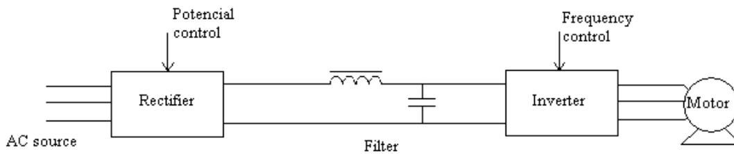
Figure 3-27: Speed control in induction motors with DC link
