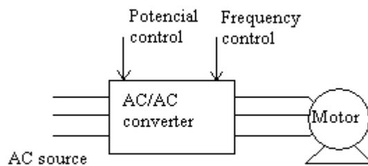
Figure 3-29: Speed control in induction motors without DC link
