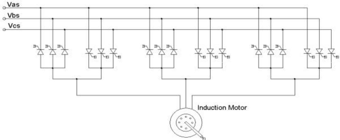
Figure 3-30: Cycloconverter induction motor drive
