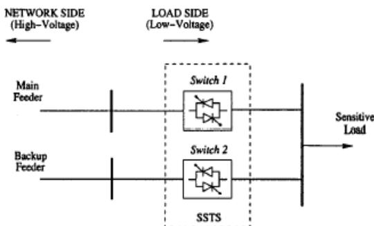
Figure 3-18: Schematic representation of the SSTS as a custom power device
