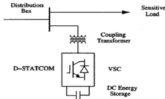
Figure 3-16: Schematic representation of the D-STATCOM as a custom power controller
