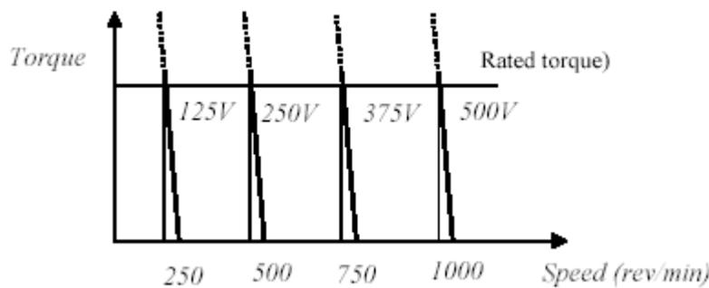
Figure 3-22: Speed-Torque characteristic in separately excited DC motor
