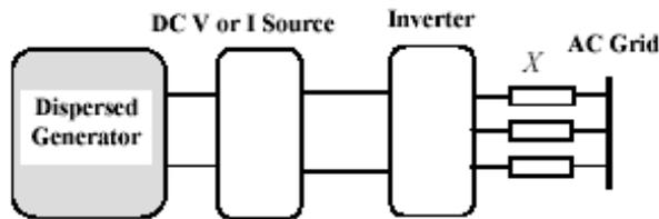
Figure 4-22: Typical converter interface to grid
