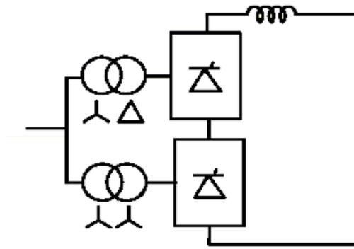
Figure 3-35: 12-pulse converter unit graphical symbol
