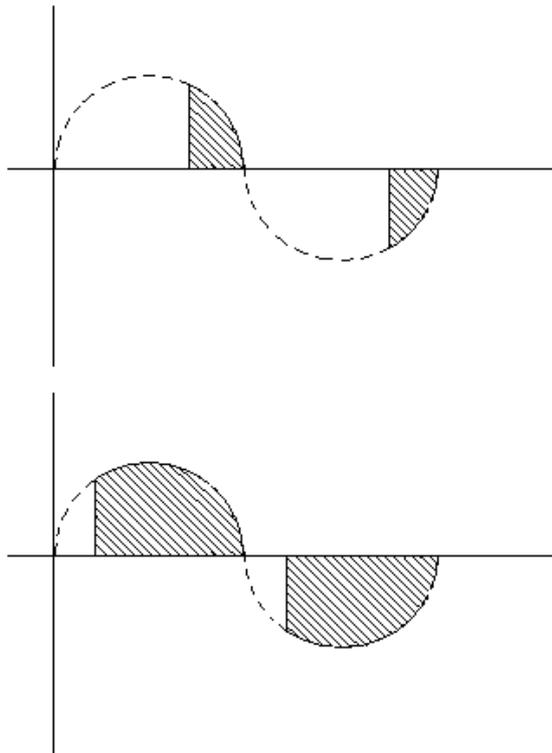
Figure 4-21: Phase cut principle of operation of the soft starter
