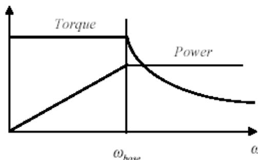
Figure 3-23: Speed regulation of a separately excited DC motor
