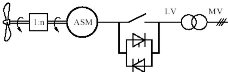
Figure 3-33: Constant speed wind turbine configuration
