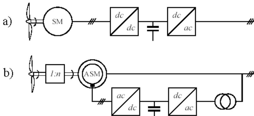
Figure 3-34: Variable speed wind turbines:
