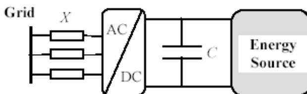
Figure 4-23: Typical converter interface to grid
