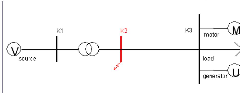
Figure 2-3a: Short circuit calculation according to IEC-909
