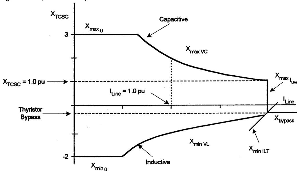
Figure 4-3: Multimodule TCSC equivalent reactance
