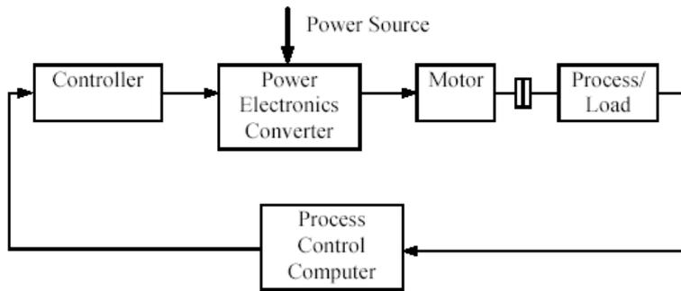
Figure 3-21: General configuration of a motor controller
